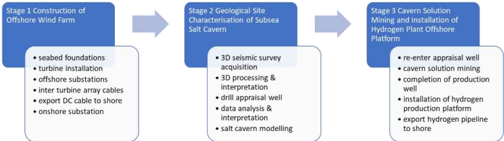
Figure 5. Offshore Green Hydrogen Production Facility Construction
