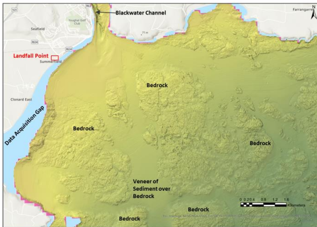
Bathymetry Map highlighting seabed features and interconnector landfall point .
